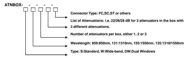
Example: ATNBOX-DW-135-3-22/26/28-SC is for attenuator box, 1310/1550nm, with 3 different kind of attenuators inside, 22dB, 26dB and 28dB, with SC adaptors.
